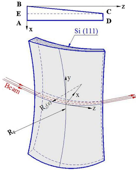
Fig. 2. The crystal deflector cut along the  $z$  axis. At the top, the cross section of a straight crystal is shown.
