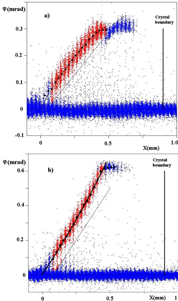
**Fig. 4.** Measurements of the correlations between  $\varphi(x)$  and  $x$  for the first crystal (a) and for the second crystal (b). An approximation of the data with a second order polynomial is shown with the solid line. Filled circles correspond to the mean value of the distribution of the events in narrow intervals of  $x$ . (For interpretation of the references to color, the reader is referred to the web version of this article.)
