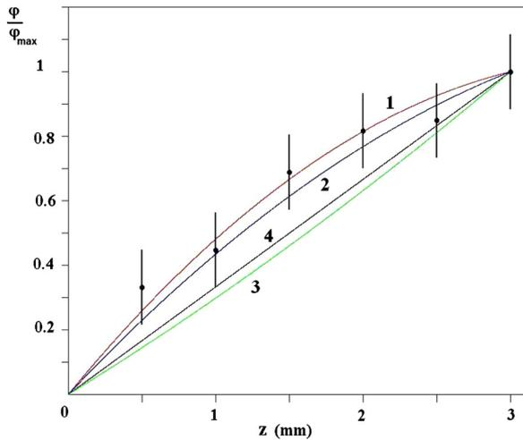
Fig. 3. The relative deflection angle as a function of coordinate  $z$ . The results of measurements for the first crystal are shown by filled circles with error bars. The curve 1 is the approximation  $\varphi(z)/\varphi_{\max} = (z - Cz^2/2L_0)/(L_0(1 - C/2))$  calculated for  $C = 0.8$ . The curves 2 and 3 are obtained by approximating the experimental data for the first and second crystals, respectively, with a second order polynomial. The curve 4 is the linear dependence ( $C = 0$ ).
