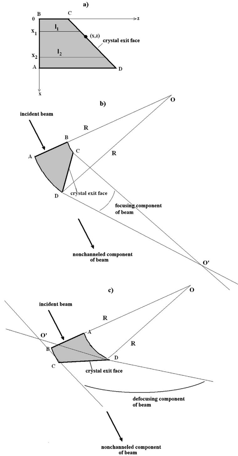
**Fig. 1.** (a) Geometry of a straight crystal, (b) the diagram showing the principle of beam focusing and (c) the diagram showing the principle of beam defocusing. Points  $O$  and  $O'$  correspond to the center of the bend and the focal point, respectively.
