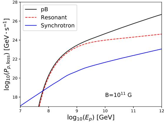
**Fig. 2.** The rate of energy loss of ultra-relativistic proton as a function of its energy. The total rate due to the  $pB$  process are shown with the black solid line, and that due to the synchrotron radiation with the blue solid line, while the red dashed line shows the contribution from the resonant interaction. The strength of the magnetic field is taken to be  $B = 10^{11}$  G.
