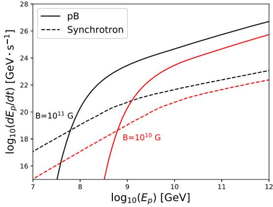
**Fig. 3.** The rate of energy loss of ultra-relativistic proton as a function of its energy in different magnetic field:  $B = 10^{10}$  G (red lines) and  $B = 10^{11}$  G (black lines). Solid lines show the rates due to the  $pB$  process, while the dashed lines show the rates due to the synchrotron radiation.
