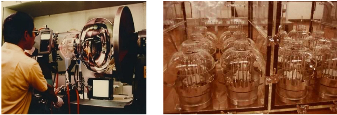
Fig. 5. Manufacture of the 20-in PMT (Courtesy of Hamamatsu Photonics K. K.).
