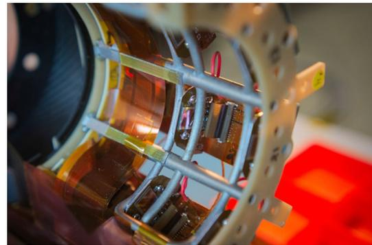
**Fig. 4** Closeup of an assembled cassette, with the gray cooling tubes visible in the foreground, the hybrid boards behind (one is visible at the center of the picture, carrying the silicon sensor visible as the silver rectangle), and the HDIs running horizontally in the background. The port card is just visible to the left of the ribbon in the foreground
