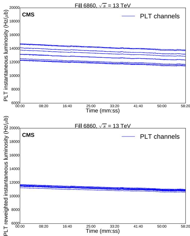
**Fig. 26** Top: PLT per-channel luminosity values as a function of time for fill 6860 in 2018, showing the total (i.e., over all BXs) instantaneous luminosity as measured by the PLT detector. Bottom: per-channel luminosity values for the same fill after applying the per-channel weights described in the text to correct for differing linearity and efficiency
