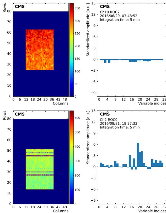
**Fig. 16** The top two plots show an occupancy map for a single ROC during a period of good operation and the corresponding values of the 31 variables used as input to the  $k$ -means clustering. The bottom two plots show similar plots for a period when the pixel data was not correctly decoded, resulting in line errors in the occupancy plot
