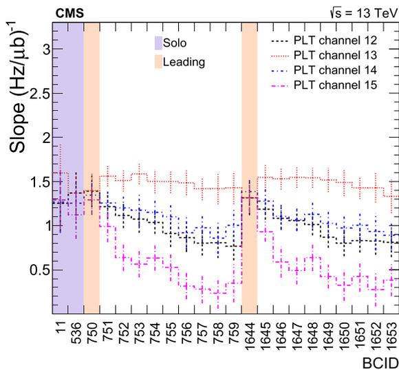
**Fig. 19** Measured slope of the PLT/HFOC ratio as a function of BCID for isolated bunches (the two bunches at the left in the blue background), leading bunches (the two bunches on a light red background), and train bunches (other bunches) for PLT channels 12–15 in the high-pileup fill 7358
