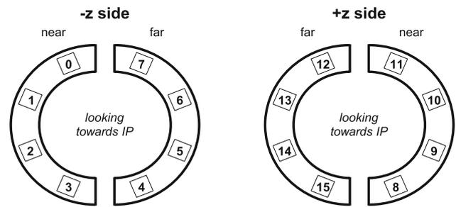
**Fig. 2** Schematic of the arrangement of the PLT telescopes, numbered by position, for the  $-z$  side (left) and the  $+z$  side (right), viewed looking towards the IP. The “near” side is the side closer to the center of the LHC ring
