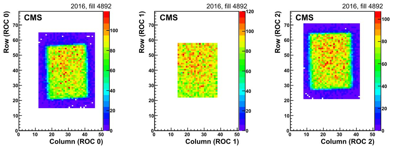
**Fig. 5** A demonstration of the active area alignment procedure in 2016, using data from LHC fill 4892. The color scale indicates the occupancy (number of hits) in each pixel. The center plane (center) uses the nor-
