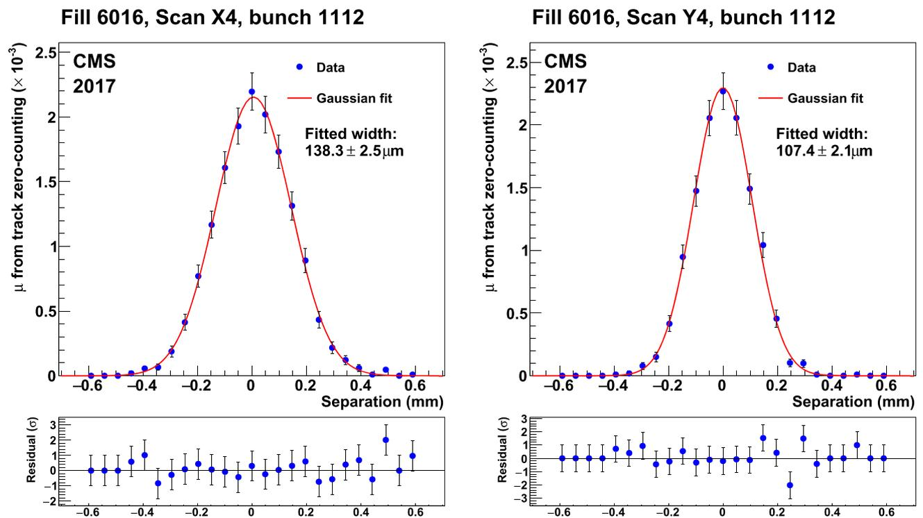
**Fig. 30** Scan curves using the track luminosity data during the fourth VdM scan pair in the 2017 VdM fill (fill 6016) for a single colliding bunch (BCID 1112) in the  $x$  (left) and  $y$  (right) directions. The extracted  $\Sigma$  and its statistical uncertainty are also shown
