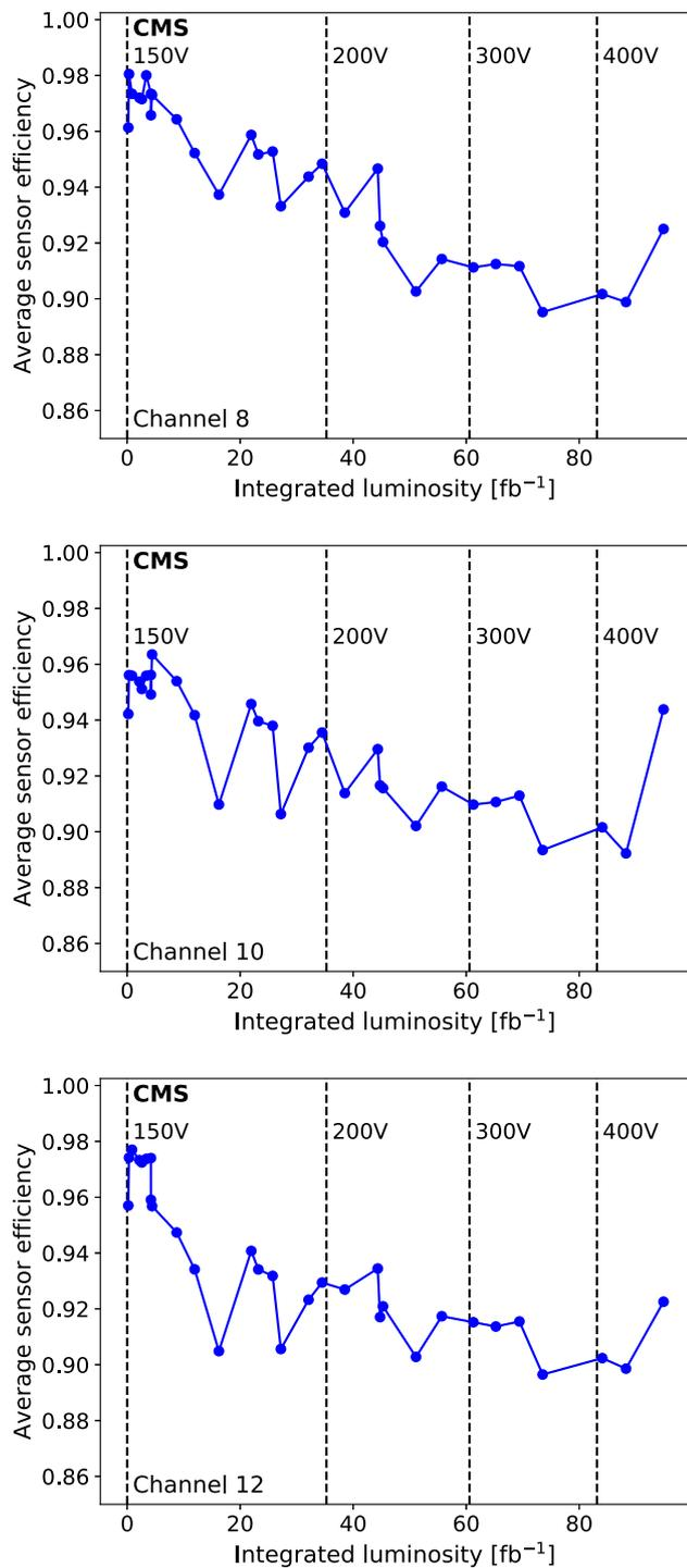
**Fig. 11** Average sensor efficiencies for three telescopes as a function of integrated luminosity in 2015–17, for channels 8 (top), 10 (center), and 12 (bottom). The dashed lines indicate points at which the bias voltage used for the sensors was changed. The uncertainties in the efficiency values are too small to be visible in this plot
