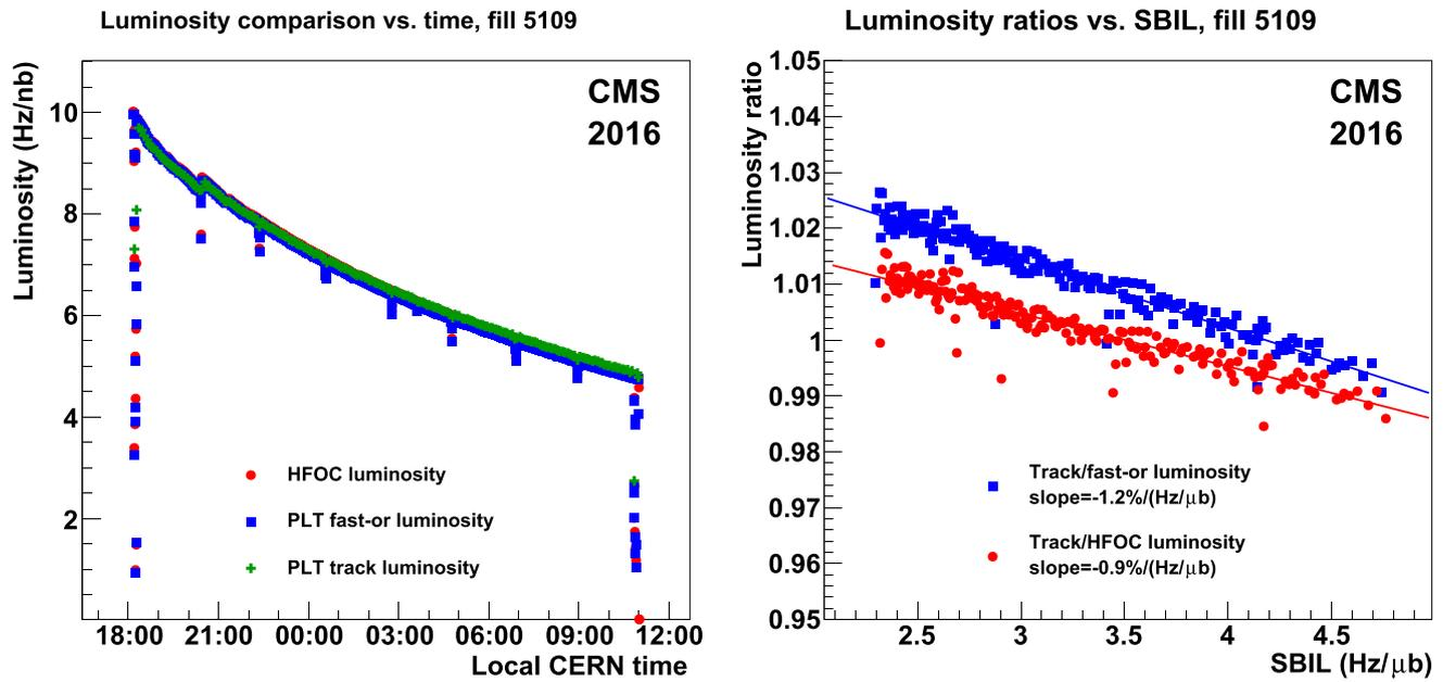
**Fig. 29** Left: luminosity obtained from track reconstruction (green crosses) vs. PLT fast-or luminosity (blue squares) and forward hadron calorimeter luminosity (HFOC, red circles) for fill 5109 as a function of time. The track luminosity is cross-calibrated to the HFOC luminosity
