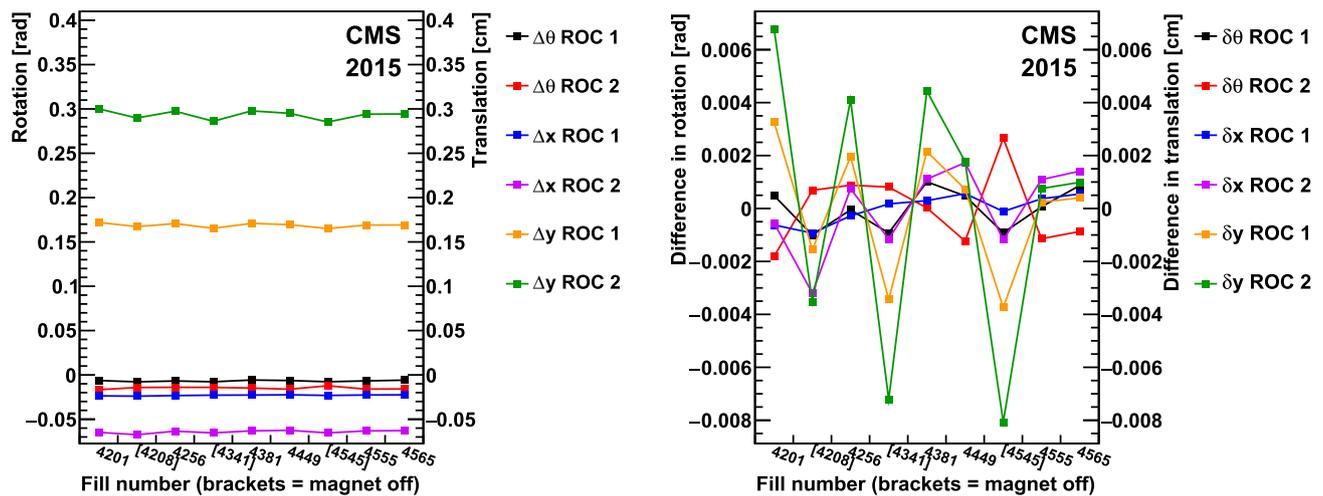
**Fig. 7** Alignment vs. time for a single PLT telescope (channel 10) for nine different fills in 2015, where brackets denote fills in which the CMS magnet was off. The alignment is described by six parameters: rotation ( $\Delta\theta$ ), translation in  $x$  ( $\Delta x$ ), and translation in  $y$  ( $\Delta y$ ) of ROC 1 relative to ROC 0, and the same three quantities for ROC 2 relative
