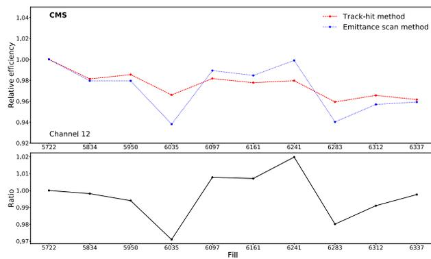
**Fig. 24** The average sensor efficiency for channel 12 obtained with the track-hit method (dashed red line) and the per-telescope efficiency measured from the analysis of the emittance scan data (dotted blue line), with their ratio (solid black line) shown in the lower pane, as a function of time in 2017. Both efficiencies are normalized to 1 for the first fill considered. The uncertainties in the individual values are too small to be visible
