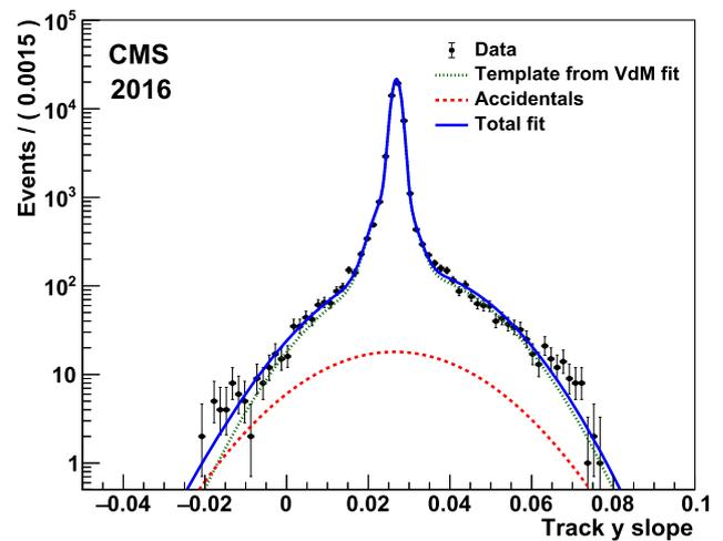
**Fig. 9** Maximum likelihood fit to the slope distribution from fill 4979 in 2016 with an instantaneous luminosity of approximately  $6 \times 10^{33} \text{ cm}^{-2} \text{ s}^{-1}$ . The dotted green curve represents the component from the distribution at VdM luminosity, the dashed red curve represents the additional accidental contribution at higher luminosities, and the solid blue curve is their sum
