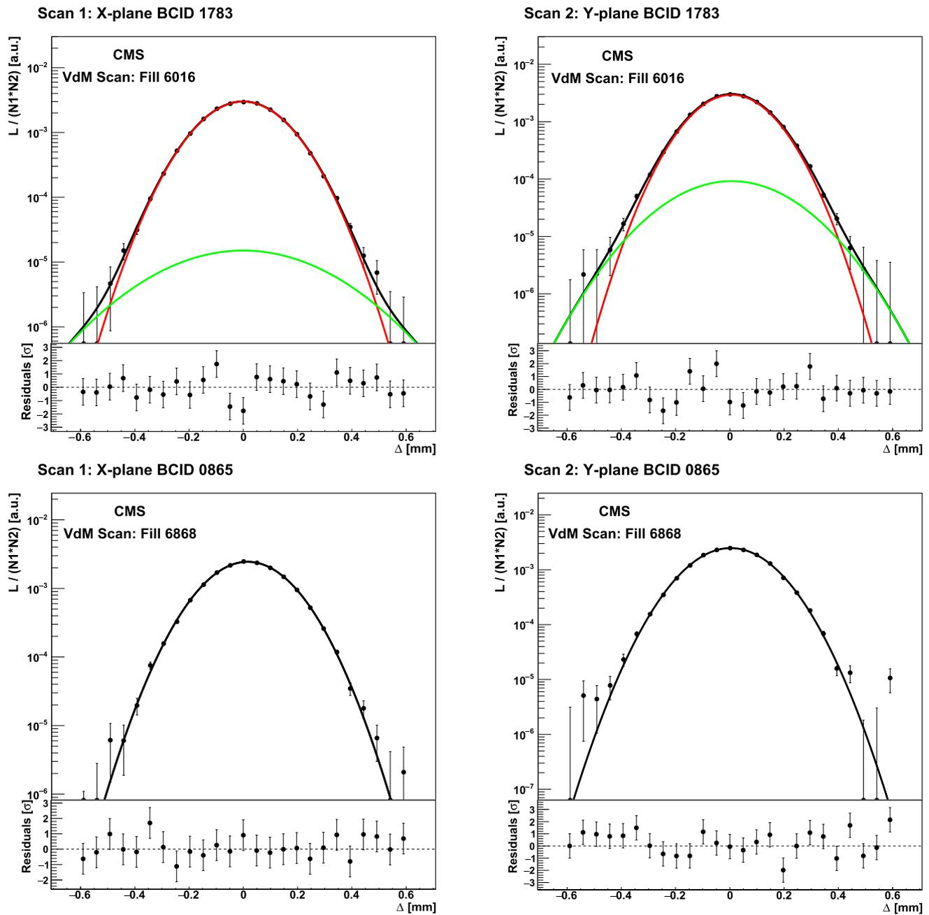
**Fig. 22** Normalized PLT rates (dots) and the resulting fitted Gaussian scan curves (black curves) as a function of the beam separation ( $\Delta$ ) for a single colliding bunch, for scans in the  $x$  (left column) and  $y$  (right column) direction. The top row shows results from a scan pair in the 2017 VdM program in LHC fill 6016 [34], using a double Gaussian fit (the two individual components are shown by the red and green curves),
