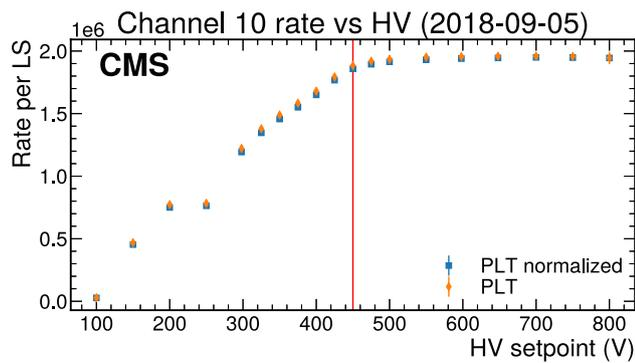
**Fig. 14** Raw (orange diamond) and normalized (blue square) rates at each HV set point for channel 10 in a 2018 scan. The vertical line indicates the calculated  $V_{\text{maxEff}}$ . We observe some nonuniform behavior at low HV values, likely due to time walk effects
