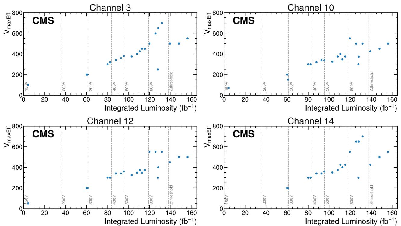
**Fig. 15** Calculated  $V_{\max\text{Eff}}$  derived from HV scans as a function of integrated luminosity for four selected PLT channels: channel 3 (upper left), channel 10 (upper right), channel 12 (lower left), and channel 14 (lower right). The dashed vertical lines indicate changes in operating
