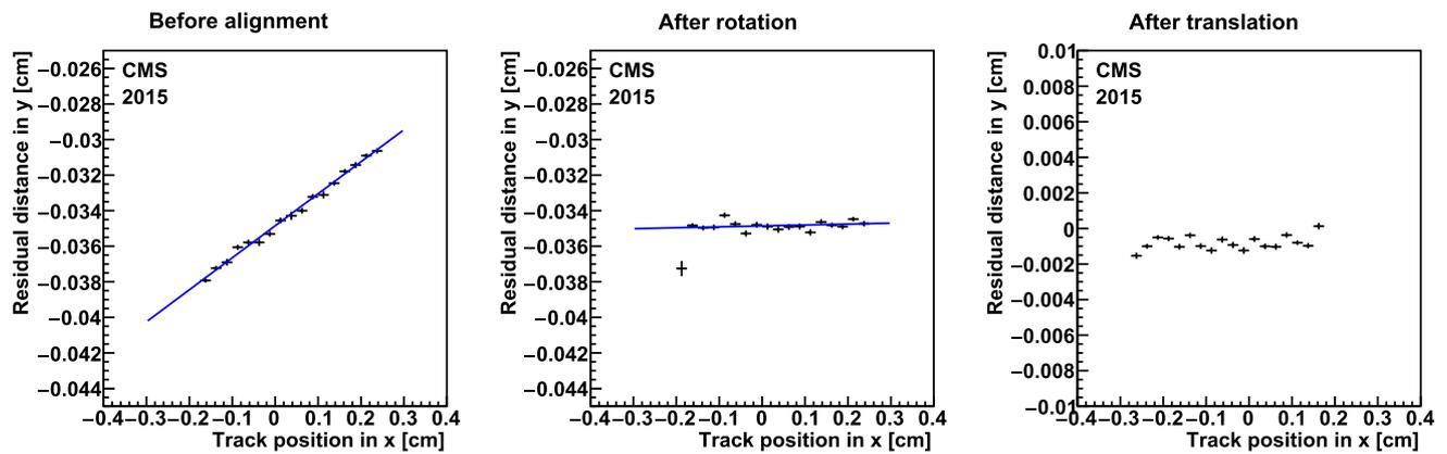
**Fig. 6** The XdY plots for the second plane (ROC 1) in telescope 7 for fill 4444 in 2015, showing the profiled distribution of the  $y$  residual distance between the hit position and the fitted track as a function of the  $x$  coordinate of the track at the plane. The three plots show the three stages of the alignment: (left) before alignment, assuming that the second and third planes are in exactly the design position relative to the first plane;
