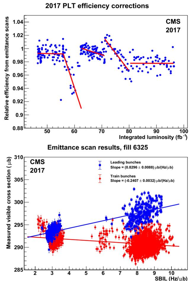
**Fig. 23** Top: efficiency corrections determined from the 2017 emittance scan analysis as a function of the integrated luminosity over the course of the year. Bottom: linearity measured for a single fill (fill 6325), showing the results from emittance scans at the beginning (right side) and end (left side) of the fill for leading (blue squares) and train (red circles) bunches. The fits for each type of bunch are shown by the lines, and the resulting slopes are shown in the legend
