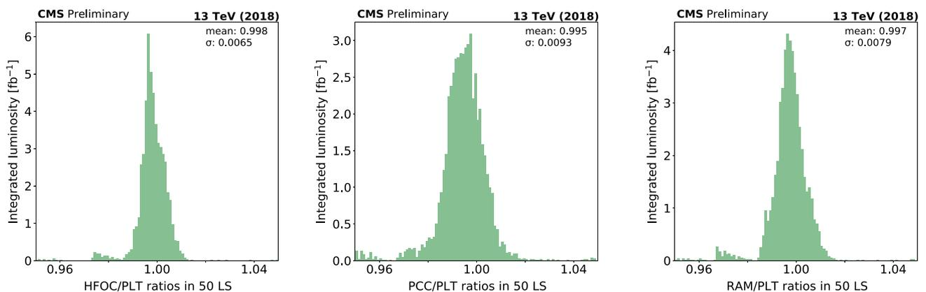
**Fig. 27** Ratio histograms for different luminometer pairs during 2018. Each entry represents a period of 50 lumi sections, weighted by the luminosity in that period. Left: HFOC/PLT; middle: PCC/PLT; right: RAMSES/PLT
