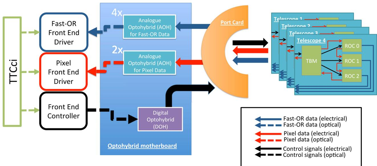
**Fig. 3** A schematic of the readout scheme for a single PLT quadrant, showing the data flow from the individual ROCs through the port card and OMB to the FEDs and FEC on the back end. The FEC and pixel FED are shared among all four quadrants, while one fast-or FED serves two quadrants
