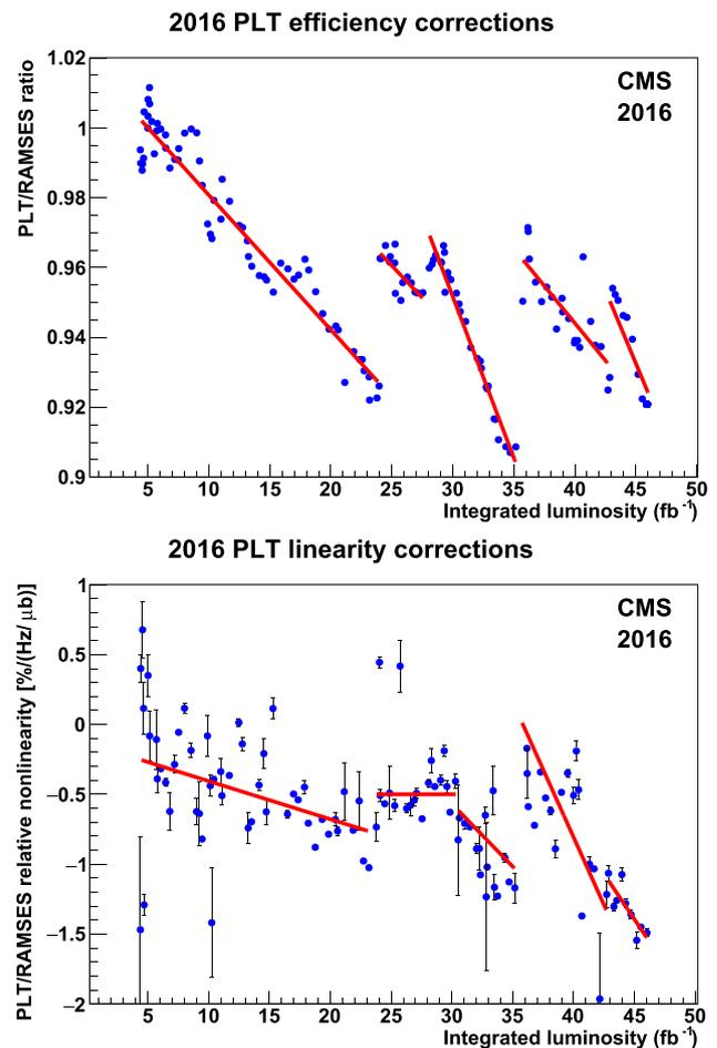
**Fig. 25** Top: efficiency of PLT relative to RAMSES over the course of 2016, where each point represents a single fill. Bottom: linearity of PLT relative to RAMSES over the course of 2016, where each point indicates the fitted nonlinearity and its uncertainty for a single fill. The red lines show the fit functions that are used to obtain the final efficiency and linearity corrections for 2016. The uncertainties in the efficiency measurements are too small to be visible on the plot
