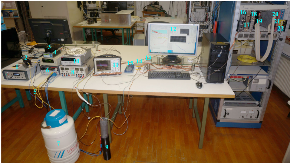
Fig. 1 Experimental setup: (1) ALPHALAS Picosecond Laser Diode Driver PLDD-20M; (2) Laser shutter; (3) Laser shutter controller (Melles Girot electronic shutter controller); (4) GOPHER power supply for the laser shutter controller; (5) Optical fiber; (6) KEITHLEY power supply for the two resistive heaters; (7) Liquid nitrogen container; (8) HAMEG power supply for the pre-amplifier of the custom electronics board; (9) Cylindrical plastic container with a radio-frequency shielding box inside; (10) KEITHLEY 6517B electrometer; (11) LeCroy oscilloscope; (12) National Instruments LabWindows
