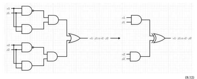
One should note that the symbol of the NAND operation (the combination of NOT with AND leading to  $a, b \mapsto \overline{a \cdot b}$ ) enters the graph
