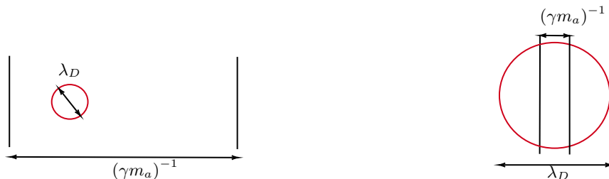
Figure 2. Cartoon depiction of scales. The domain wall, of plasma-frame Lorentz-contracted width, L \sim (\gamma m_a)^{-1} , is shown between the two vertical lines. The red circles depict the size of the Debye sphere - the scale at which collective modes respond. Left Panel: in this case, the wall thickness is much larger than the Debye scale. Right Panel: the opposite case where the wall thickness as seen in the plasma frame is smaller than the Debye scale.
