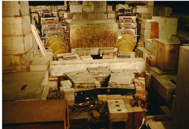
Fig. 13. Shielding arrangement with roof open.
