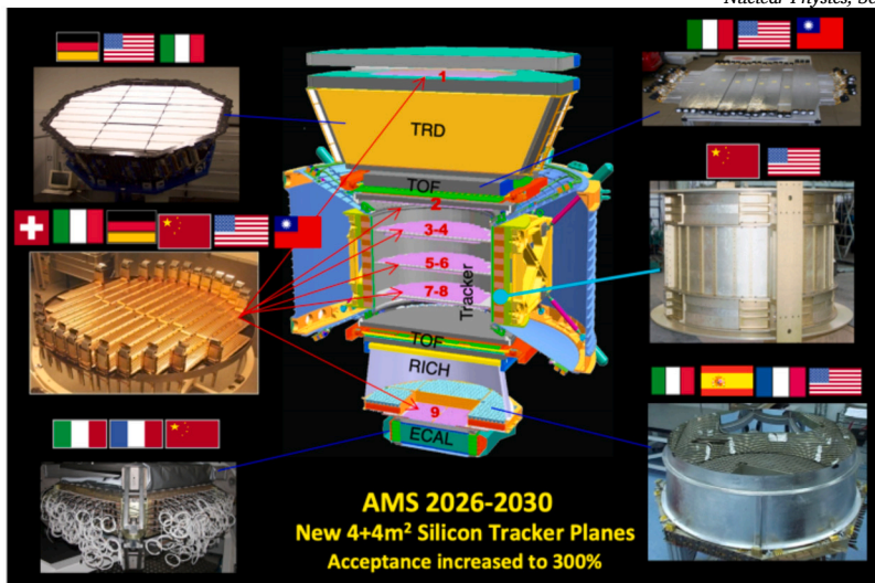
Fig. 36. Layout of the AMS experiment showing the countries which participated in the construction of individual detectors.
